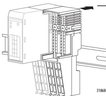
3. Press firmly to seat the mounting base on the DIN rail until the mounting base snaps into place.
