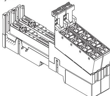
2. Rotate the terminal block into the mounting base until it locks itself in place.
