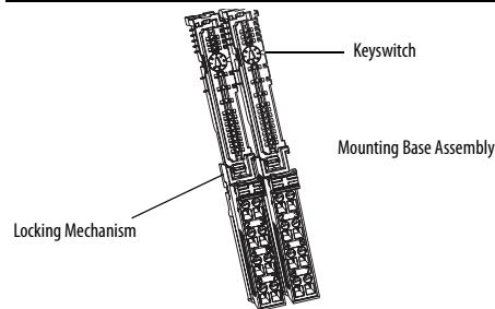
2. Verify the DIN rail (orange) lock screw is in the horizontal position. You cannot insert the module if the mounting-base locking mechanism is unlocked.
